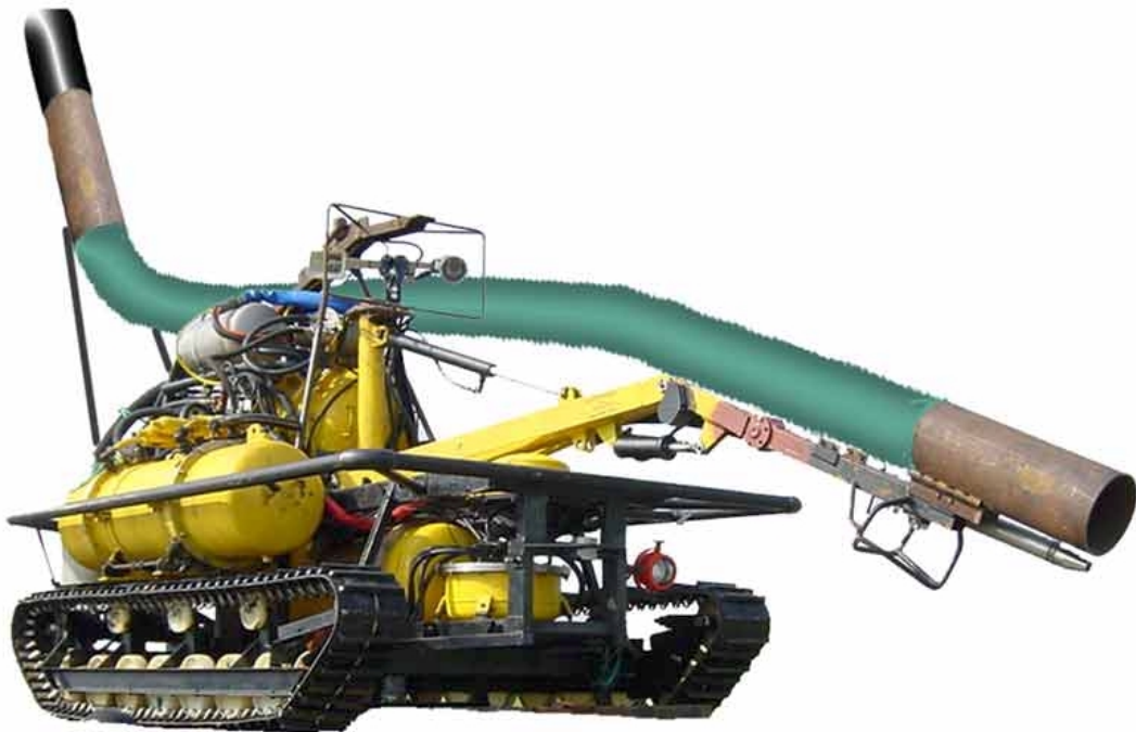
SBD2 at it's current configuration, fitted with an water jet and airlift on the manipulator.
