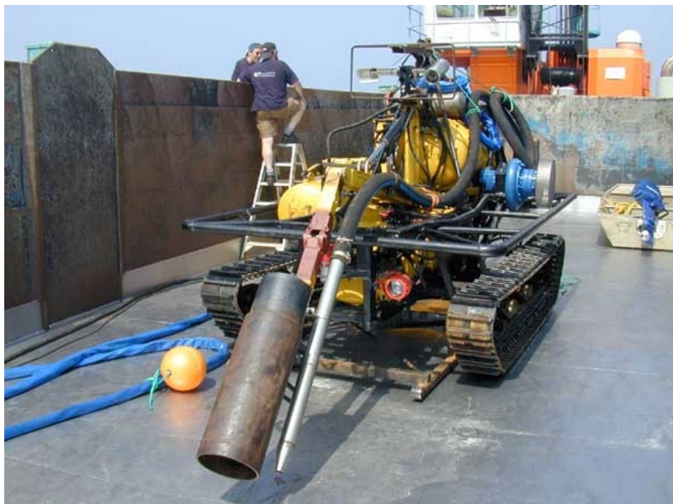
The Seabed dredger ready for a test run in Holland. The SBD2 is fitted with a water jet, 125 m 3 /hr.-900kPa and a 10" airlift(hose not mounted) on the manipulator. On top you can see the pan & tilt unit with a color zoom video camera and a light.
